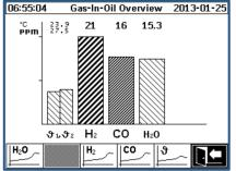
Individual chart diagram for Hydrogen ( $H_2$ ), Carbon Monoxide (CO), Moisture in Oil ( $H_2$ O) and temperatures.
